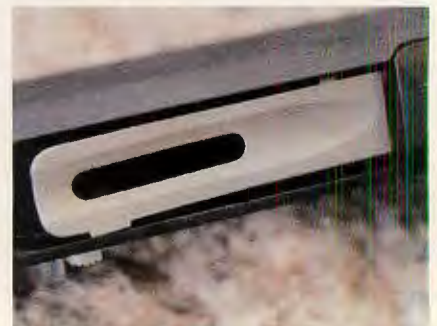
BELOW: MAG-10's slotted shell lifter should've helped clear testers' several stoppages, but the shell-stop didn't hold rounds after they were pried back into the magazine tube.
